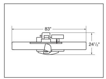
Figure 8. Minimum working clearances.
